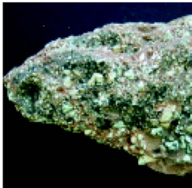
Pebble conglomerate with sandstone from Boley, Okfuskee County. This rock, which is called the Boley Conglomerate, is a member of the Vamoosa Formation, an important aquifer in east-central Oklahoma.
