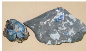
Chert (white and gray) that contains the mineral galena (blue-gray). The smaller sample contains sphalerite (dark red) and galena (blue-gray). Found near Picher, Ottawa County.
